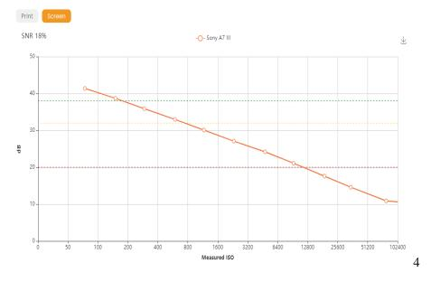
There are no discontinuities in the SNR plot. Since both the signal and SNR lines are straight, the noise line must also be straight, almost constant. Nevertheless:
