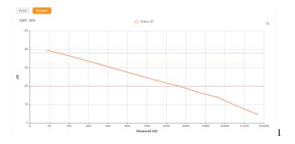
The vertical scale is in decibels (dB). Note that the change in SNR is almost linear.
