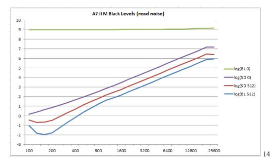
There is no discontinuity but there is something else happening at the low ISO range. The SD value is higher than the average value after subtracting 512 for the black level. The distribution of noise around the average is not a normal SD bell curve because the raw values (not the log values) cannot go below 0.
