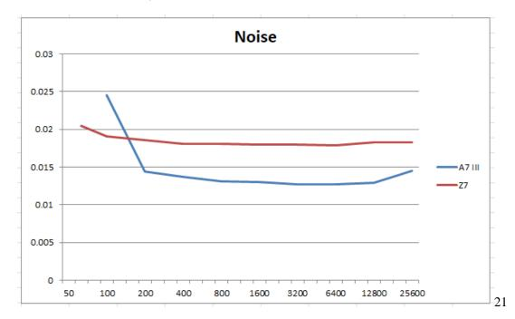
It implies that the noise does not change with ISO except at the top and bottom of the ISO analog range. It bears no resemblance to the plot of the black levels for the two cameras in images 12 and 13.
