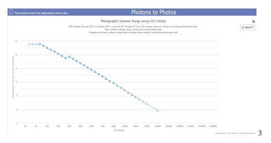
The P2P plot narrows down the break in linearity to between ISO 320 and 400.
