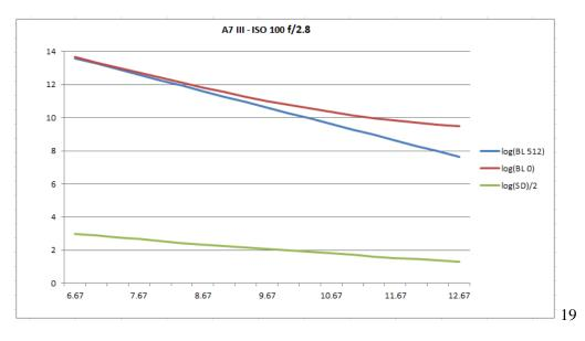
The blue line is the plot of base 2 logarithm for middle gray after subtracting the black level of 512. DxO shows the SNR for middle gray in decibels (dB). Converted to base 2 logarithms:
