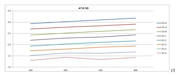
By over and underexposing the target we can obtain these results to plot of the SD for the A7 III:
