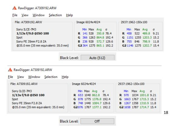
The average raw values and SD ( $\sigma$ ) were recorded for the two green channels. The test was run at base ISO by varying the shutter speed.
