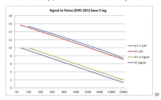
If we use the signal from the middle gray value and the SNR from DXO we can calculate the noise assumed by DXO.
