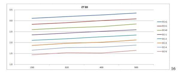
These are plots of the standard deviations. Discontinuities are not as pronounced as they are in the read noise plots because the assumed noise is higher than the read noise itself.
