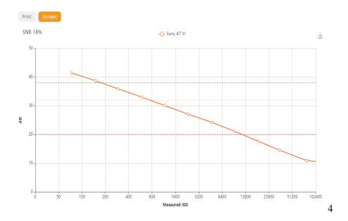
There are no discontinuities in the SNR plot. Since both the signal and SNR lines are straight, the noise line must also be straight, almost constant. Nevertheless:
