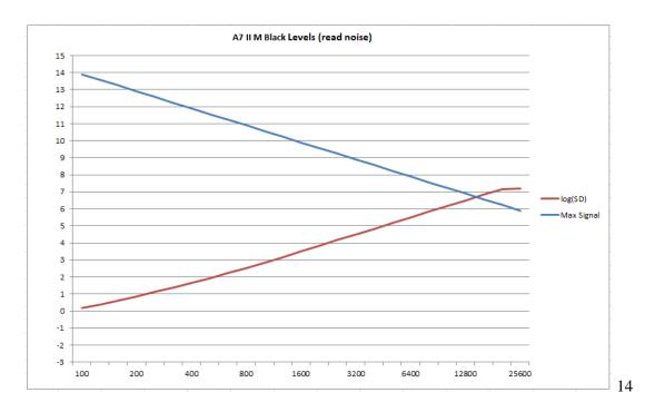
There is no discontinuity but the final SD value looks wrong so the analog range might end at ISO 20000. By over and underexposing the target we can obtain these results to plot of the SD for the A7 III:
