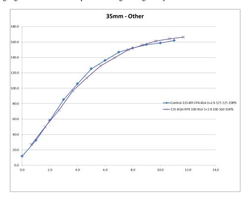
It's not an exact match but it tells me what I needed to know. The film can be used at ISO 160 and developed in Xtol 1+1 for a little more than 8 minutes (8.5?) to get what I want. It took only one roll to figure out the ISO and development time.
