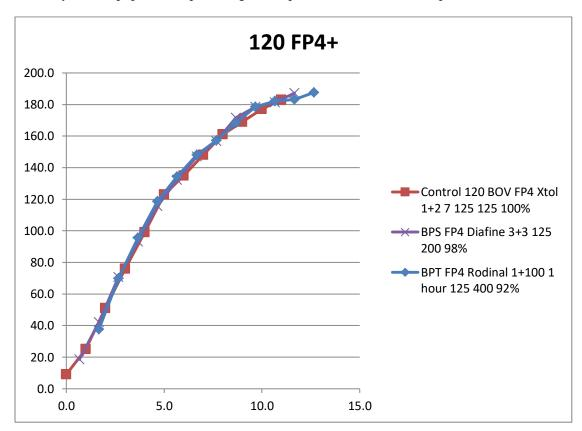
Because of additional development in the shadows, both methods allow you to expose at higher ISO settings (lower exposures). In this case, FP4 can be used at ISO 200 in Diafine or ISO 400 with Rodinal stand development. Each approach may require a change to the scanner gain adjustment or a selection of a softer grade of paper but neither one alters the fundamental shape of the characteristic curve.
