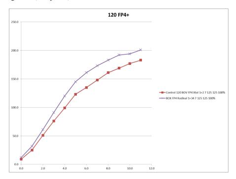
It's not that far off. But to get the same curve as the control an adjustment to both the ISO and development time is appropriate. Using ISO 160 and a gain adjustment of 90% the result looks like this:
