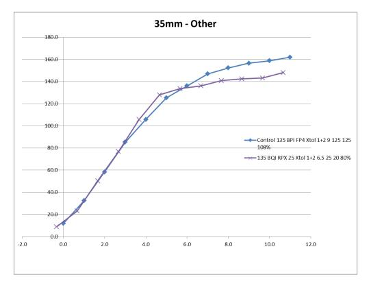
The shape of the curve is peculiar and resembles CMS 20. It looks normal up to middle gray and then the contrast drops abruptly. The same thing happens with different developers and concentrations so I know that it's a characteristic of the film. I can try to match the film to a scene where I want this to happen but the problem with both films is that they are very thin and curly – not worth the trouble.
