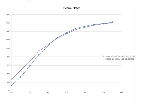
The highlights look OK but the left end of the curve shows that the shadows would be overexposed. So I adjusted the ISO to 160 and got the shadows to line up:
