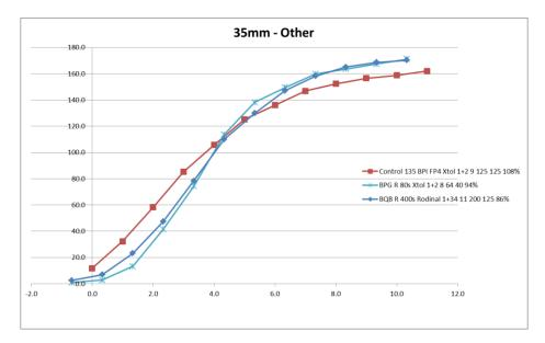
Both of these films have very low FB+fog but the curling is well controlled. They have higher contrast in the mid-tones and lower contrast in the shadows and highlights but the change is gradual and they capture most of the 11 stop range. I ended up rating them at ISO 40 and 125 and the test show that they need more exposure and less development than I gave them initially.
